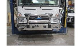
· Carefully open doors to ensure they do not hit bar at fully open. Re-adjust product if required.
